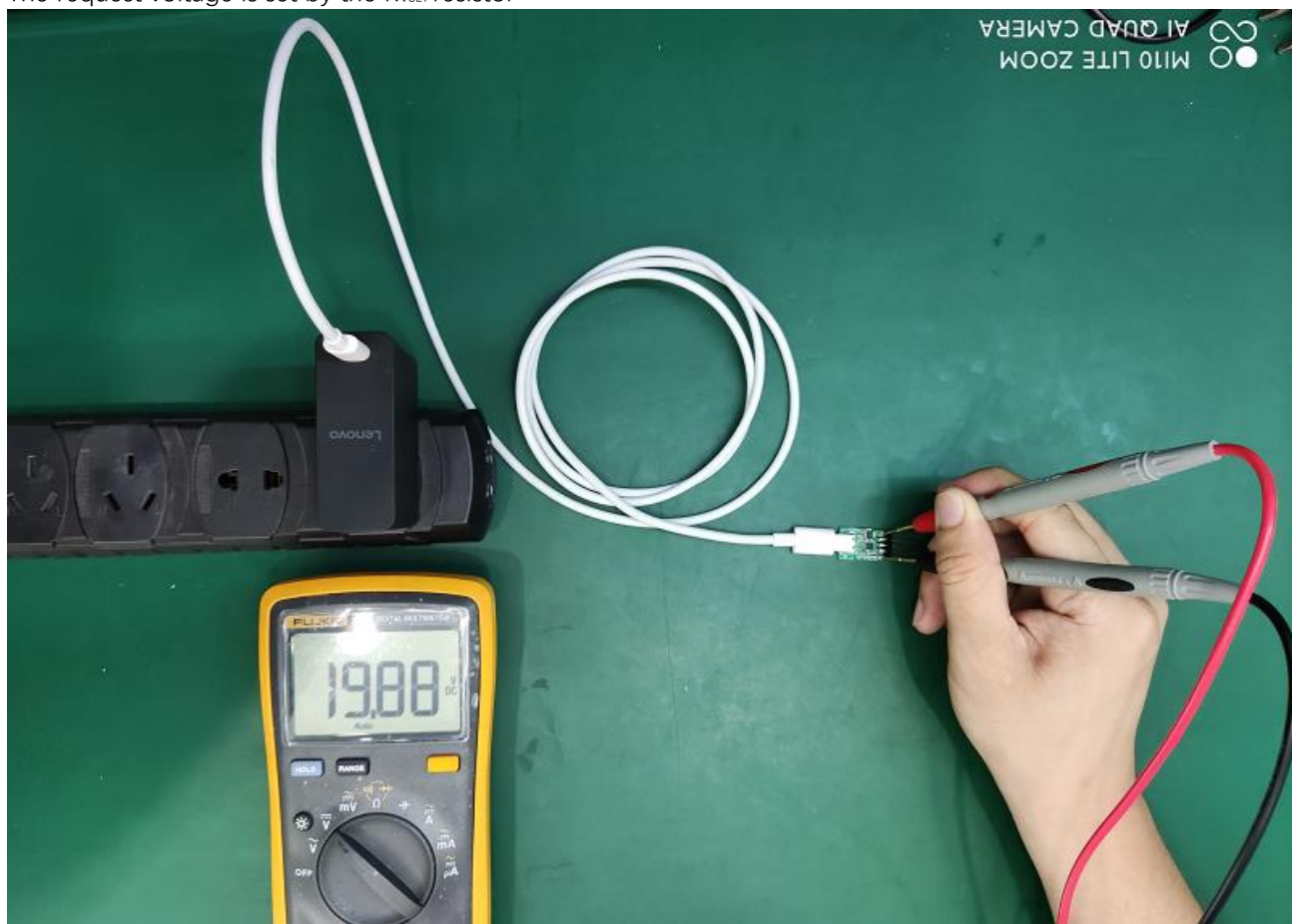
Figure 5. EVB Tested by R VSET and R ISET Resistors
